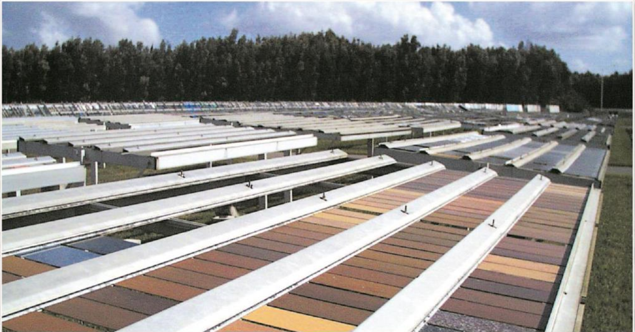
Pict. 1: Florida test exposed samples
